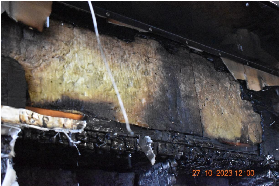
Photo No. 30 Test specimen after the test. Insulation between the fire chamber and the flame deflector.
