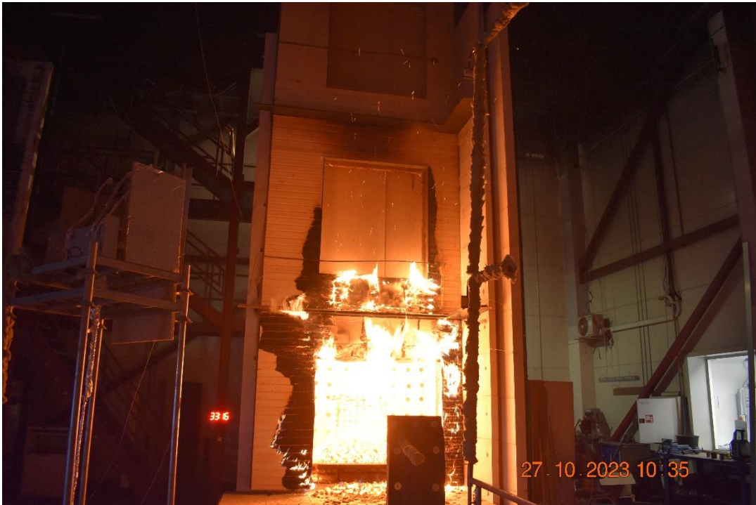
Photo No. 23 Test specimen 33 minutes into the test.
