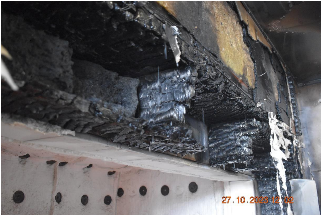
Photo No. 33 Test specimen after the test. The cassette above the fire chamber.
