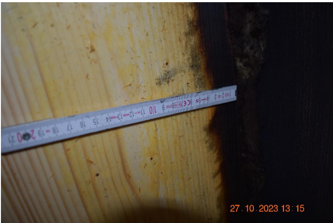
Photo No. 36 Test specimen after the test. Cassette at the right side of the first window.
