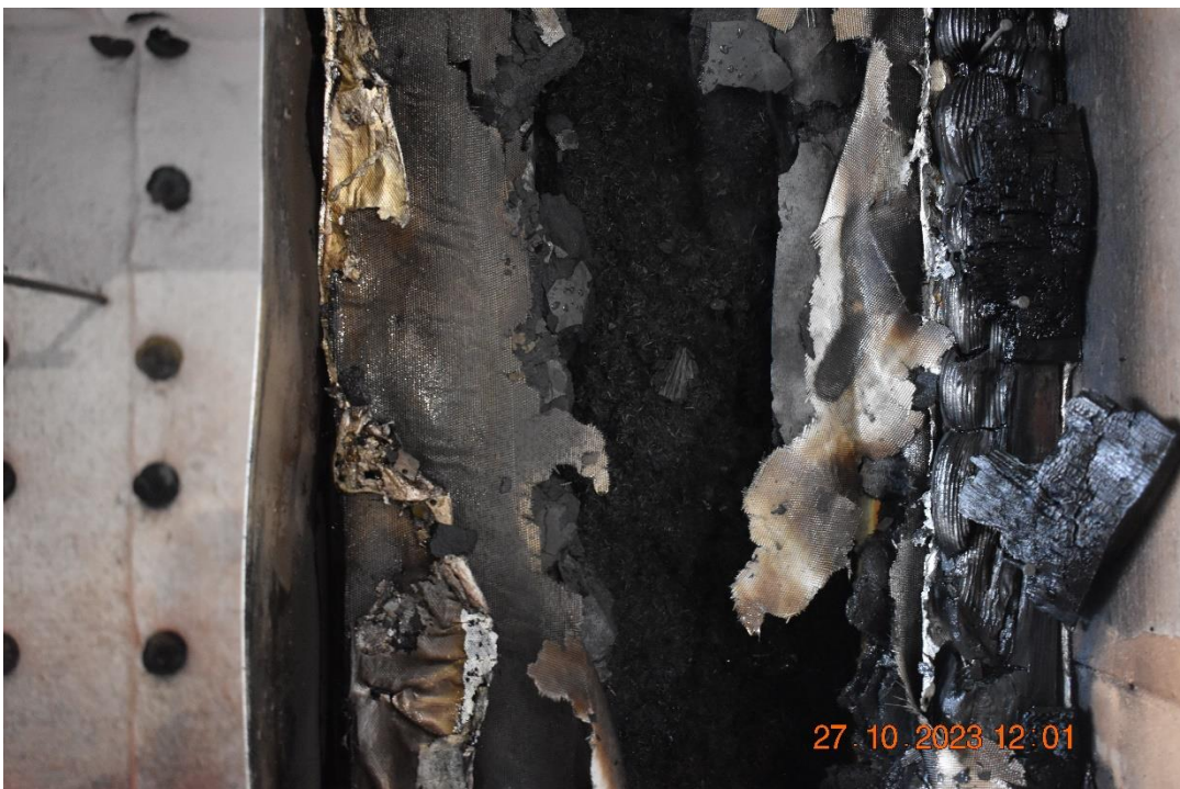
Photo No. 32 Test specimen after the test. Detailed photo of the left side of fire chamber.
