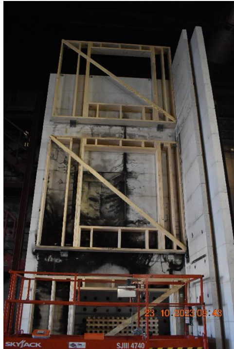
Photo No. 1 Prefabricated cassettes mounted on the façade rig.
