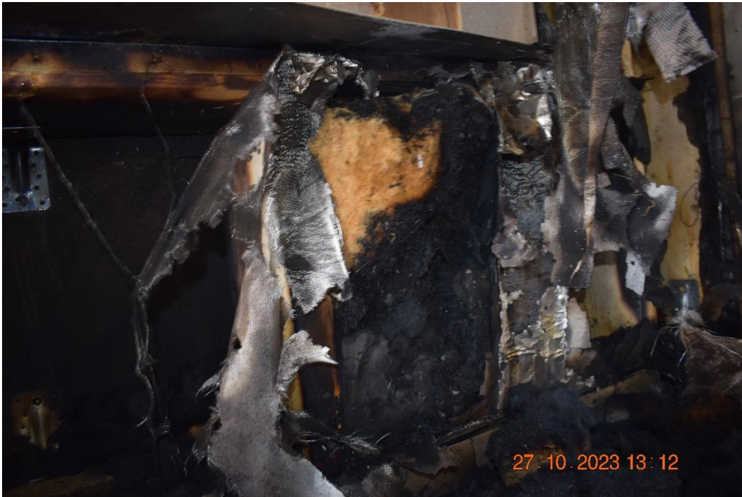
Photo No. 35 Test specimen after the test. Insulation at the bottom of the first window.
